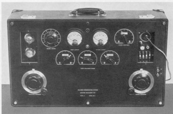
FIGURE 1. Front view of the CBS antenna measuring set
