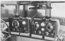
The interior of field car No. 3 showing the signal generator unit at the left and a receiver at the right. The hand wheel for orienting the loop is shown at the top of the photograph
